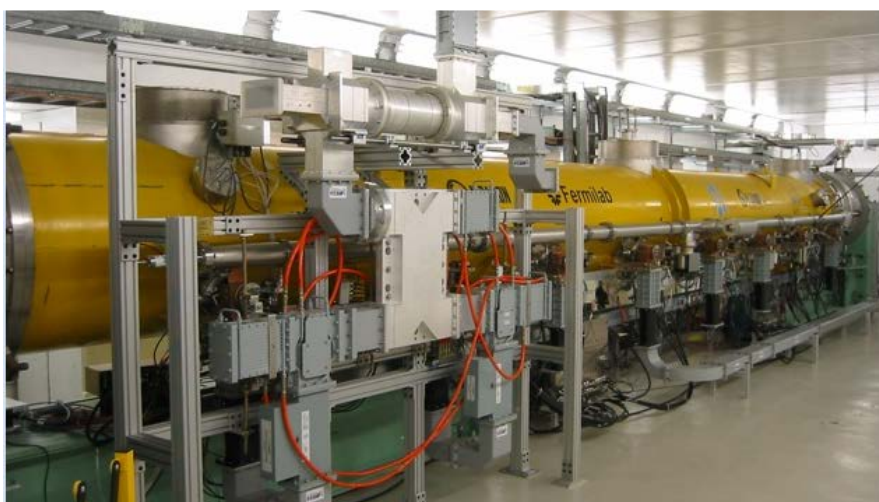
Figure 6: The first 1.3 GHz SRF cryomodule installed in the ASTA facility.
