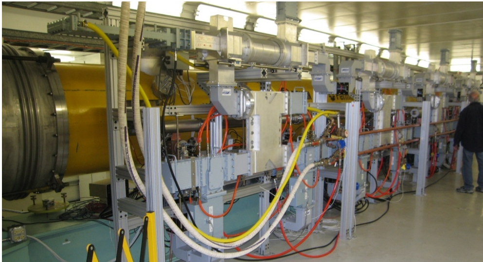
Figure 6: Photograph of cryomodule I installed in the ASTA beamline enclosure. View is looking downstream. Waveguide distribution structure is on the right of the cryomodule.
